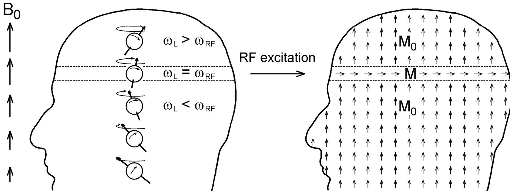
A magnetic field gradient is applied during the RF excitation pulse
