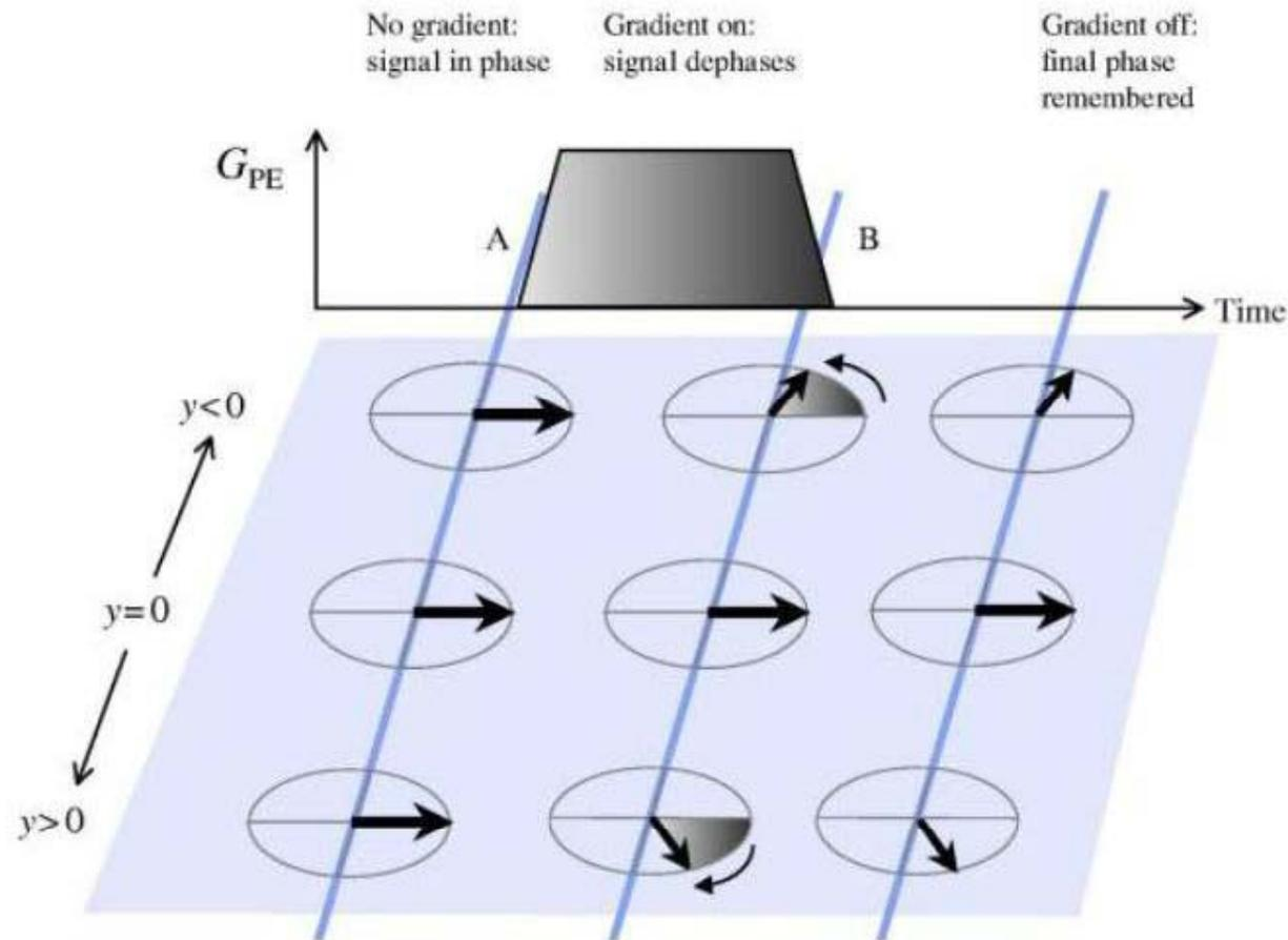
A magnetic field gradient is applied in the remaining direction for a short period **after** excitation but **before** data acquisition
