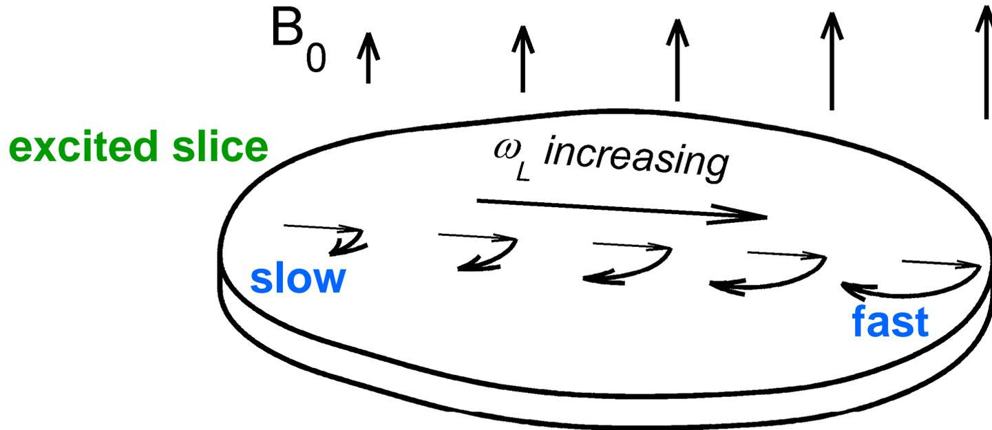
A magnetic field gradient is applied during the data acquisition
