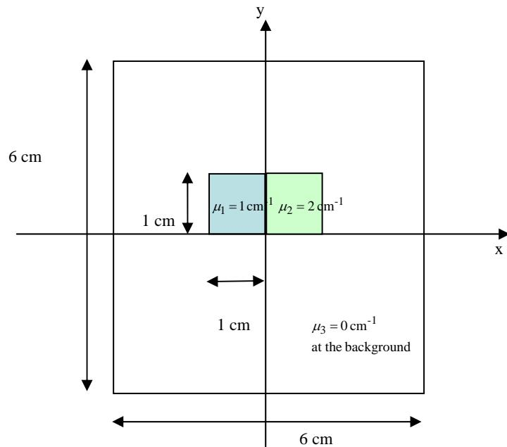
8. (10 pt) A 2-D slice to be imaged is shown in Fig. P7, which consists of two regions with linear attenuation coefficients  $\mu_1$  and  $\mu_2$ . The background has a linear attenuation coefficient of  $\mu_3$
