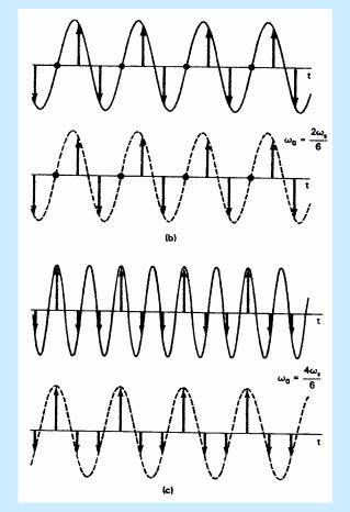
Aliasing: The reconstructed sinusoid has a lower frequency than the original!
